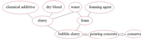
Fig. 2. The production process of foam concrete
