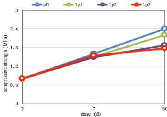
Fig. 3. The influence of chemical additive on the compressive strength of foam concrete
