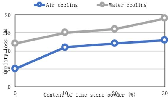
Fig. 5. The influence of chemical additive on the quality loss of foam concrete
